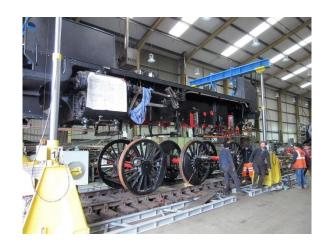
Now lower the frames onto the axles, fiddling the axleboxes and springs into position and putting some nuts on to keep everything in place.
