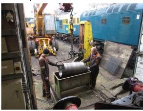
With the loco rolled out of the Goods Shed to provide better access, the liner spends some minutes in a bath of liquid nitrogen, and when John has confirmed that the liner is the right size,
