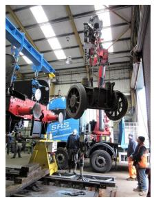
Then roll the whole lot backwards on the tracks the jacks stand on, and remove the pony truck from under the front end, using a convenient crane on a lorry.
