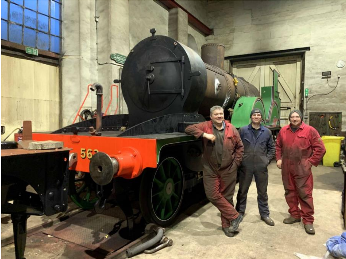
The engineers at the Flour Mill Workshop pose with the boiler test-fitted in the frames.
