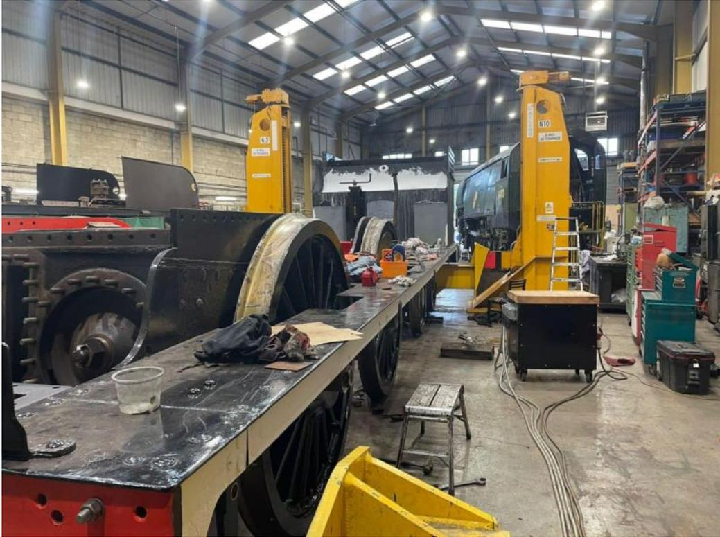
Following on from the Herston Works stuff in the previous edition of Swanning Around, we find that *Manston* has regained its wheels and has released the lifting jacks such that the M7 30053 has now got its wheels too.
