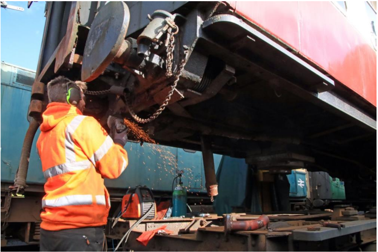
Last time we saw Alan English and Will Rudge lifting a coach on the jacks outside the Goods Shed at Swanage. This time, we see Alan carrying out repairs to the steam heating pipework.
