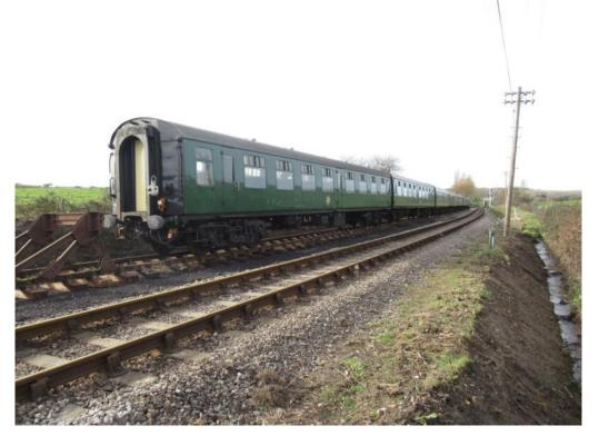
Another job undertaken by the P'Way Track Team during January was the extension of Herston siding 1 by two track panels, 60 feet each, to increase storage space. It can now take up to seven coaches and a goods brake van, as shown here.
