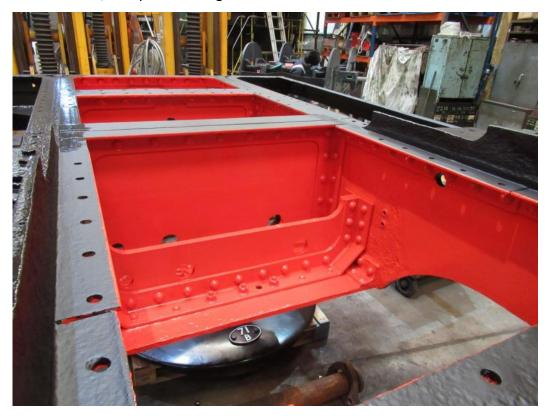
Work on the frames is complete, including new stretchers (crossmembers) having been made and fitted where the bogie attaches. (bogie = truck for our North American readers!)
