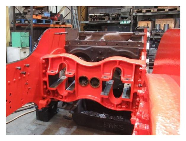
At the front of the frames, the refurbished slide bars, below, are ready to fit, but the cylinders themselves are awaiting attention and some new piston heads, castings for which are in progress.
