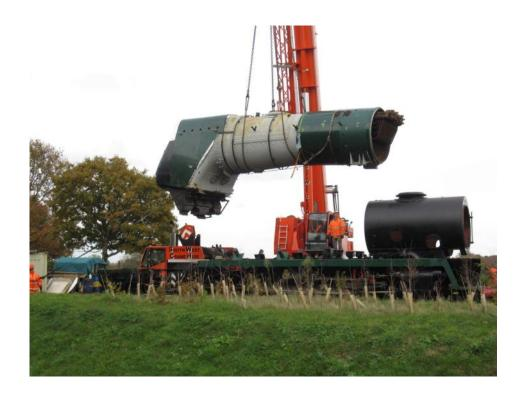
Being unable to lift the boiler into the frames of 34028 *Eddystone* in the car park at Herston, to avoid damage to the tarmac, the rolling chassis was moved from Herston on the S A Smith trailer which brought the M7 (see page 2), the boiler moved by lorry from its previous location, and the pair reunited at the RRI using a large crane.
